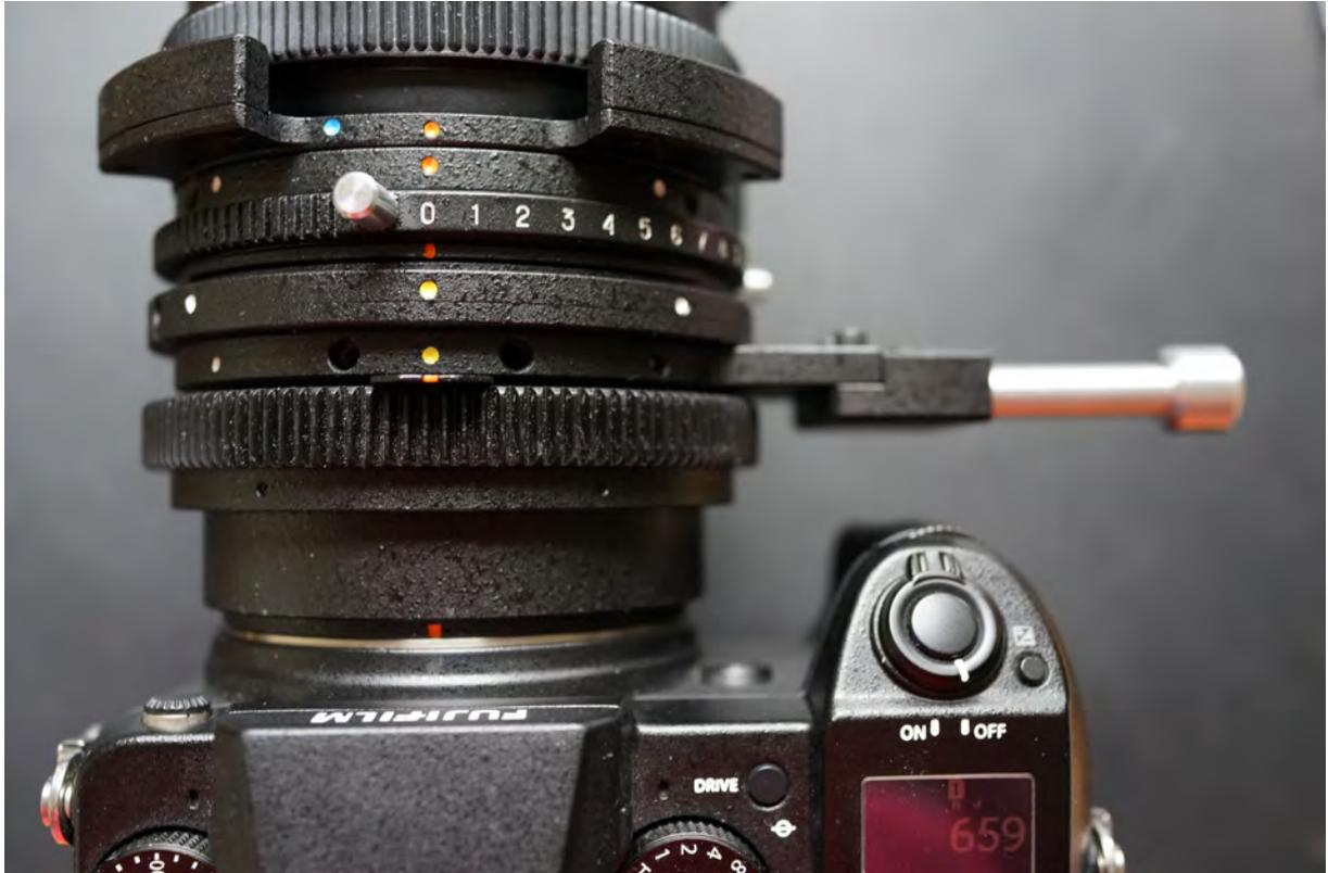
Using the white pins you may shift the lens by rotating the ring marked from 0 to 12 mm
