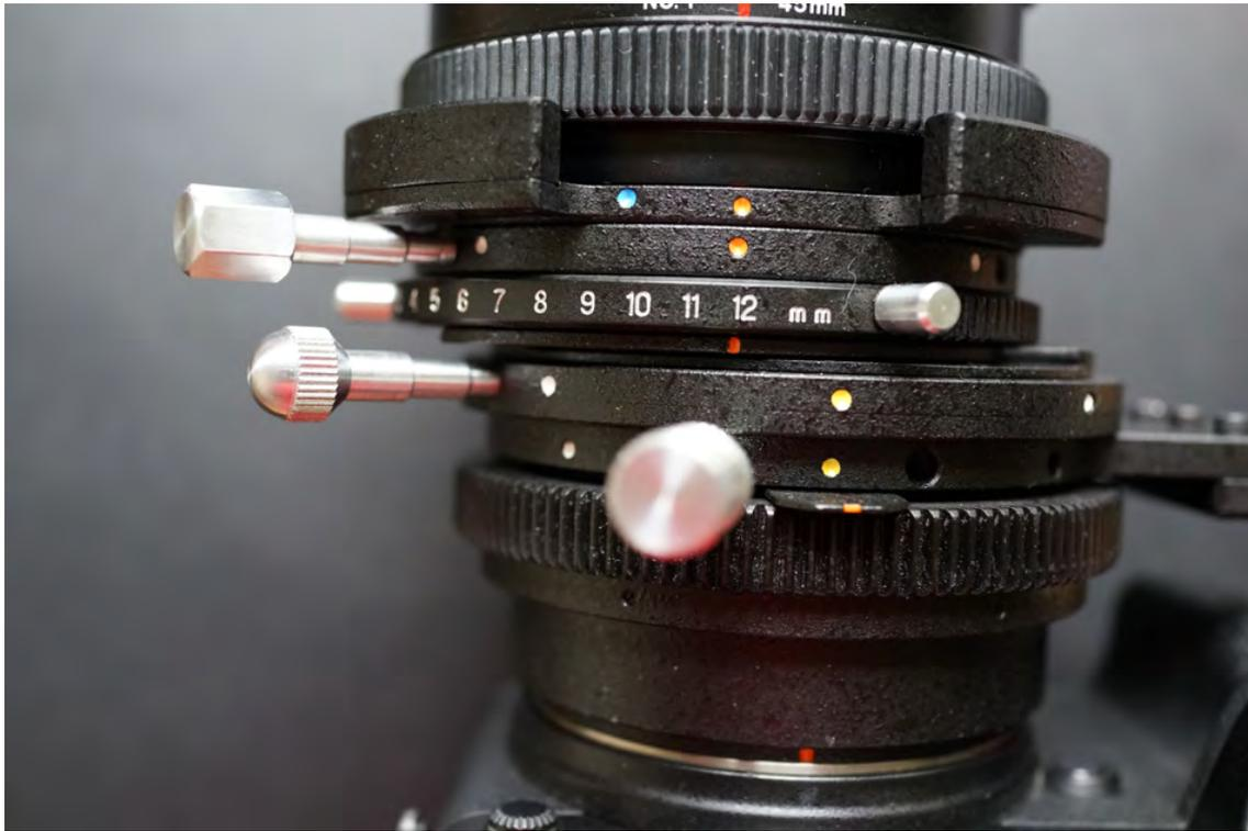
The stopping screw with the “sphere” head shown below is responsible for the rotation of shifting mechanism, therefore after you have chosen the position of the grip tool it must be always tightened up in all procedures whereas the other two stopping screws must be loosened.
