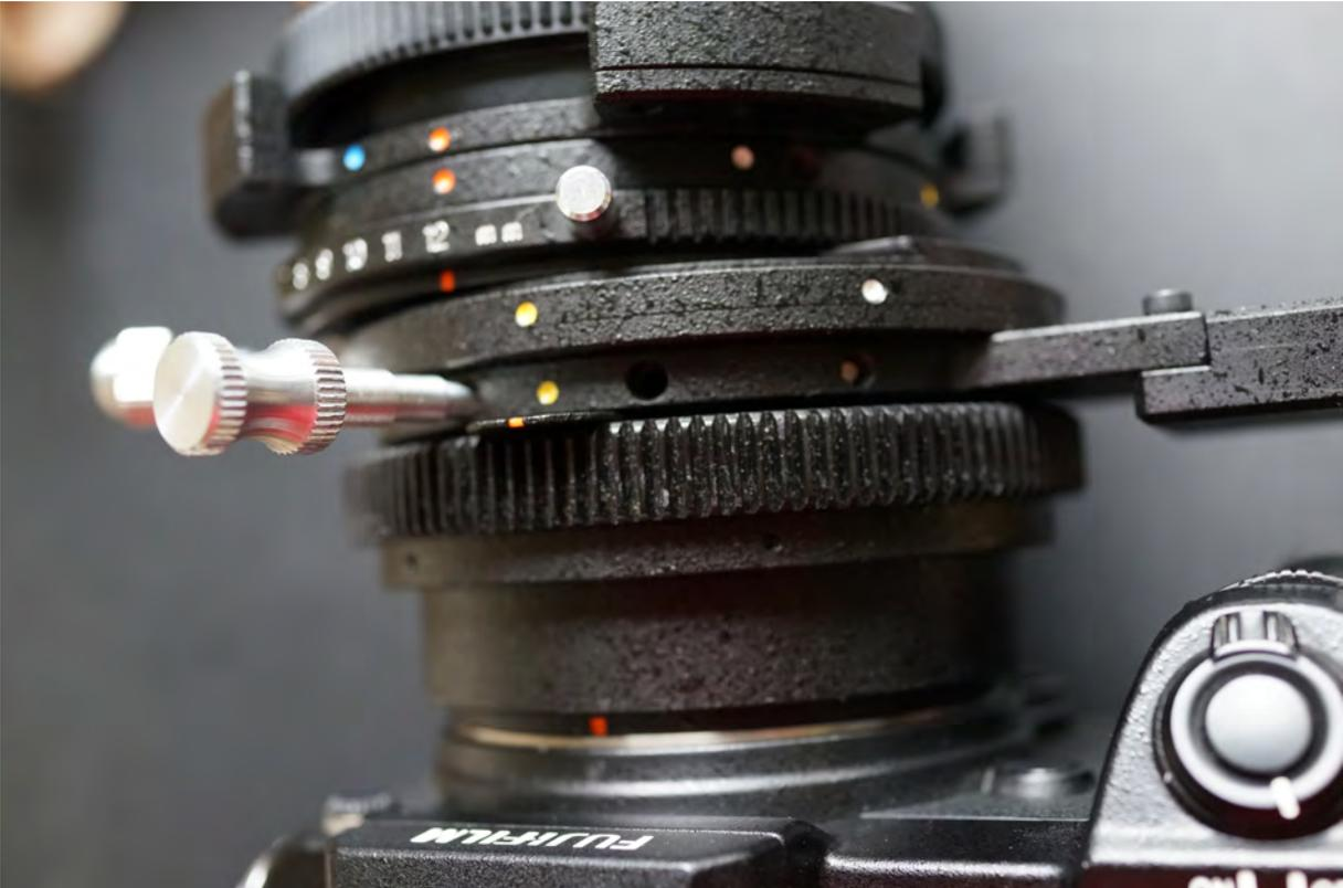
The screw with the hexagon head shown below is responsible for the lens rotation.
